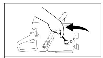
STEP 1 Loosen side cover nuts and remove side cover.
